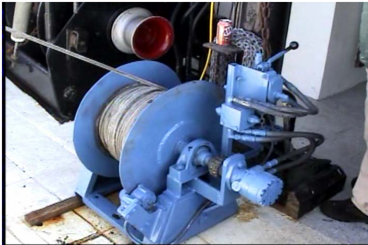
b. Oceanographic winch outfitted with electromechanical cable and slip ring
