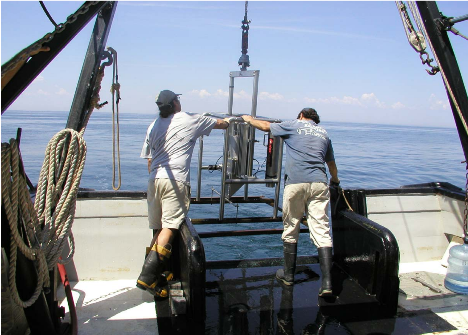
Photograph 2.7-1 CR Environmental employee, Christopher Dunbar, and Michael Cole of SAIC deploying REMOTS Camera off the F/V Christopher Andrew
