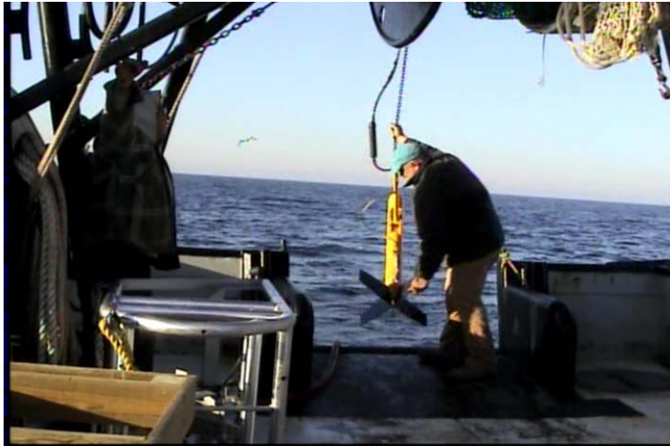
a. Chip Ryther of CR Environmental deploying the Edgetech side-scan sonar towfish
