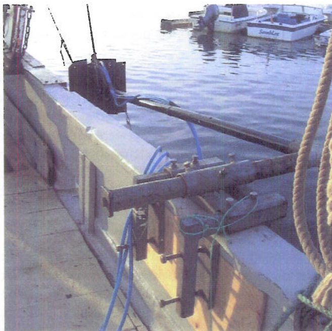
Figure 3.3b - GeoSwath transducer array mounted on adjustable boom on port side of F/V Christopher Andrew
