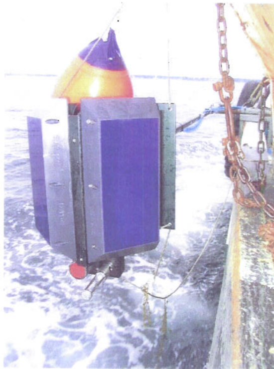
Figure 3.3a - GeoSwath V-Plate transducer array.
