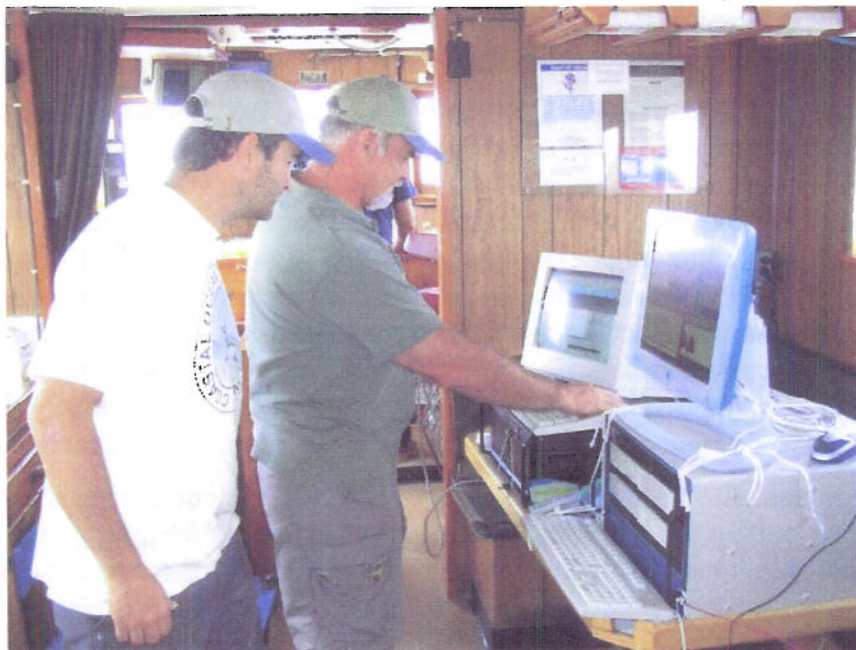
Figure 3.3c - GeoSwath topside acquisition system (right) and towed side scan sonar acquisition system (left) installed in galley of F/V Christopher Andrew.
