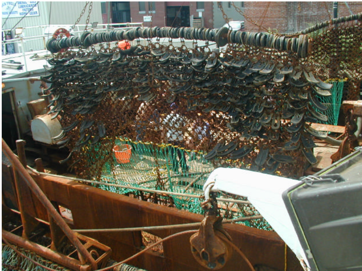
Figure 9. Club stick and chafing gear attached to the rear of a scallop dredge.
